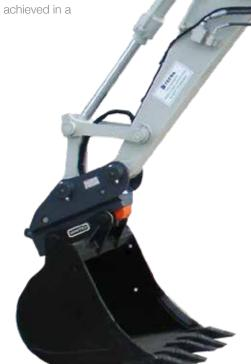
The boom configuration is unique and allows the TB2150 to function like Takeuchi's smaller excavators. Maximum versatility on sites when working in tight spaces – no more constant machine repositioning – simply use the offset both left and right (77°/53°).
