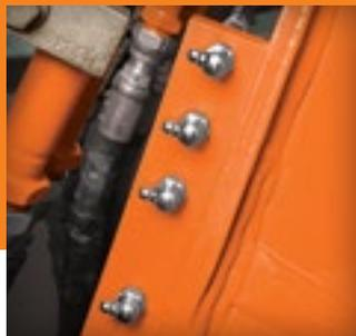
Centralized lube banks place engine oil, fuel and hydraulic pilot oil filters are all located on the same side at ground level for easy servicing.
