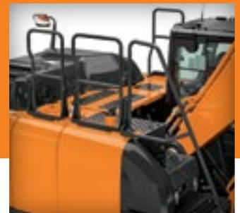
Upperstructure handrails provide added safety when servicing the engine compartment, and a larger hood gives you better engine accessibility.
