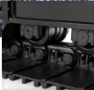
■ With large idlers, rollers and struted track links, the sealed and lubricated undercarriage is built for the long haul.
