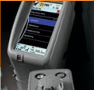
■ Multi-language LCD monitor and rotary dial provide easy access to machine info and functions. Turn and tap to select work modes, monitor maintenance intervals, check diagnostic codes and set cab temperature. Control oil flow and toggle between dig and thumb modes with a programmable thumb attachment mode.
