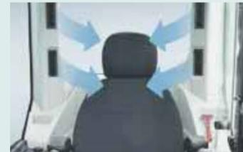
The large air-conditioner has registers on the back pillars that blow from behind and to the right and left of the operator's seat. They can be adjusted to put a direct flow of cool/warm air on the operator, which means a more comfortable operating environment.
